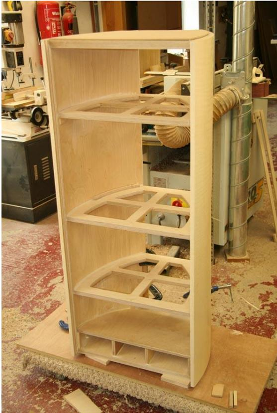
Next stage was the internal bracing and sloped internal base. Each brace had to be individually cut and shaped to ensure a millimetre perfect fit so this was very time consuming. Part of the issue is that the formers used for the side panels were hand-made and had minor inconsistencies, so if done again, CNC cut formers would be used.
