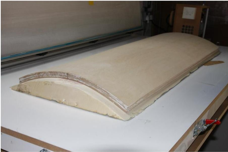
One of the side panels being laminated from multiple ply layers in a DIY vacuum former using high grade PVA glue. The glue was selected to be "lossy" so that it never sets hard but remains slightly flexible. Another way to win the battle against unwanted resonance!
