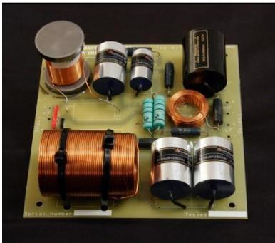
Capacitors are (all bar one) Clarity Cap ESAs. Inductors are from Janzten, the LF and notch filter inductors are air-cored although that's probably overkill. I was careful to ensure electrical compatibility with the originals, so the DC resistance measures EXACTLY as per the Tannoy originals. I had to add a resistor to the notch filter inductor (in series) to achieve the 2.6Ohms required. PCBs are custom built and fit the space for my removable panels at the rear of the speakers.
