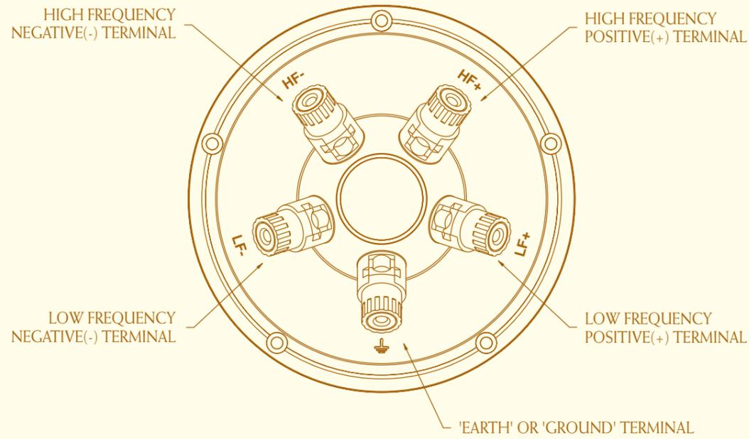
FIGURE 2: Single Wire Mode and Earth (Ground) Lead Connection
