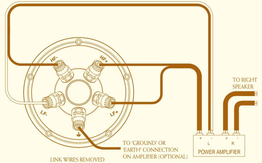
FIGURE 4: Bi-Amping Mode and Earth (Ground) Lead Connection
