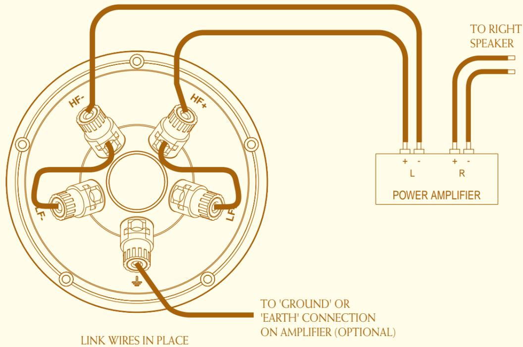
FIGURE 3: Bi-Wire Mode and Earth (Ground) Lead Connection
