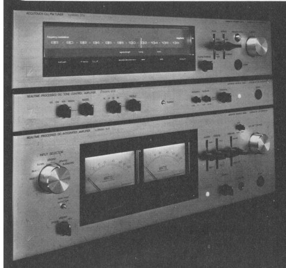
Luxman 5T10 Tuner: Features Lux's exclusive "Accutouch" tuning system. Has switchable i.f. bandwidth: wide (normal) and narrow. Signal strength indicator has five LED's. Tuning circuit employs Lux's closed-lock-loop. Audio multipath monitoring through speakers. Output level adjustable from 0 to 1 volt. Usable sensitivity, 10.3 dBf (1.8 uV); 50-dB quieting sensitivity, 14.2 dBf (2.8 uV). Capture ratio, 0.8 dB (wide i.f.).
