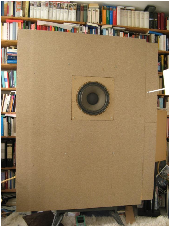
Figure 1 Measuring a Tannoy HPD 315 on a DIN baffle with calibrated microphone using MLS & time windowing
